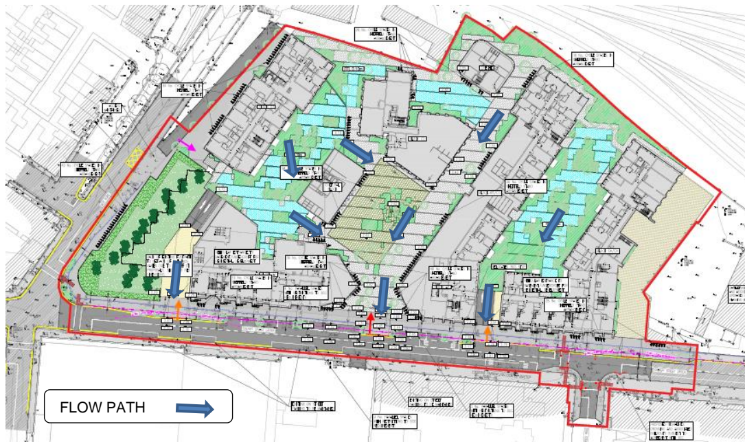
Figure 5-2: Overland flow path
